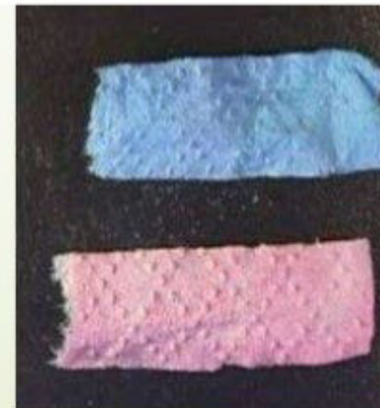
Blue cobalt-chloride paper turning pink in the presence of water
