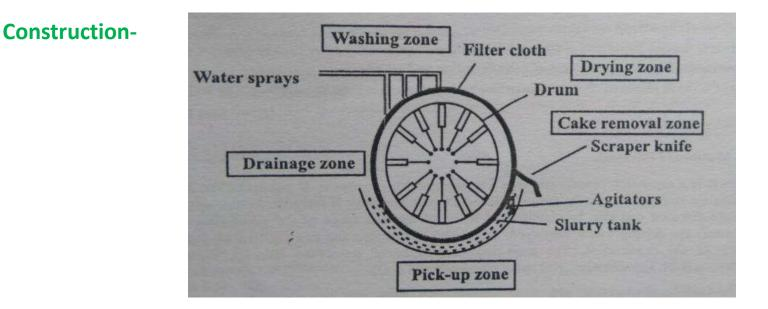
$\succ$  It consists of a metal cylinder mounted horizontally.
