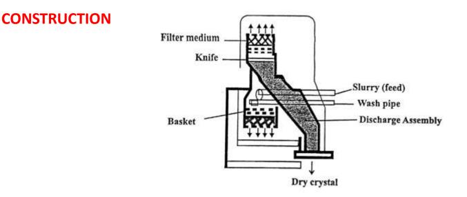
➢It consist of perforated basket mounted on horizontal shaft and run Continuously by motor.
