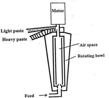
➢It consists of a long, hollow, cylindrical bowl of Small diameter and rotate on vertical axis.
