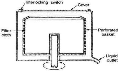
>It consists of a basket made up of steel or any other suitable metal
