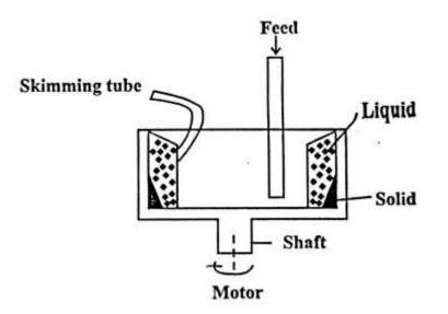
>It consists of a non-perforated basket made of steel.
